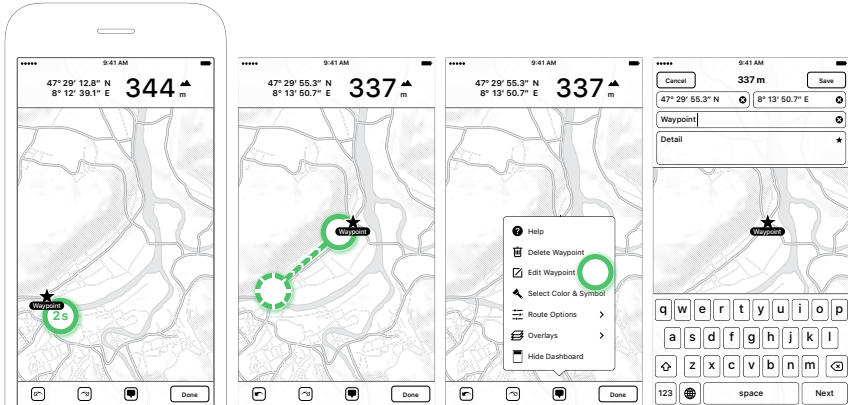
Figure 2.17: Adding a new waypoint by tapping > 2 sec – Move the waypoint by dragging it over the map – Modifying the name or detail of the waypoint – Entering the exact coordinates or title and detail information
